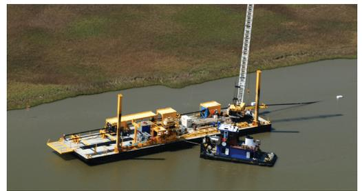
The CM14 is a combination pipelay and construction barge that effectively services most inland areas due to its 4' shallow draft.
